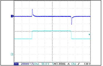
Figure 6: Output voltage response to step-change in input voltage (nominal to maximum input voltage), at Full Load current. Load cap: 15 µF tantalum capacitor and 1 uF ceramic cap. Ch 1: Vout, Ch 2: Vin.
