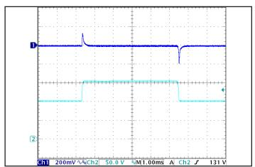
Figure 6: Output voltage response to step-change in input voltage (nominal to maximum input voltage), at Full Load current. Load cap: 15  $\mu$ F tantalum capacitor and 1  $\mu$ F ceramic cap. Ch 1: Vout, Ch 2: Vin.
