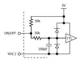
Figure B: Internal ON/OFF pin circuitry
