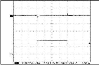
Figure 5: Output voltage response to step-change in load current (50 % -75 % -50 % of Iout(max); dI/dt = 0.1 A/ $\mu$ s). Load cap: 15  $\mu$ F tantalum cap and 1  $\mu$ F ceramic cap. Ch 1: Vout, Ch 2: Iout.
