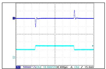
Figure 5: Output voltage response to step-change in load current (50 % -75 % -50 % of Iout(max);  $dI/dt = 0.1~A/\mu s$ ). Load cap: 15  $\mu F$  tantalum cap and 1  $\mu F$  ceramic cap. Ch 1: Vout, Ch 2: Iout. (5 A/div.)
