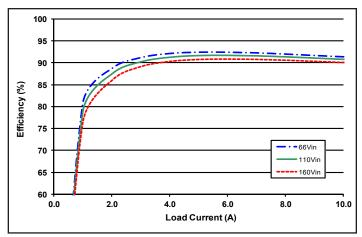
Figure 1: Efficiency at nominal output voltage vs. load current for minimum, nominal, and maximum input voltage at 25  $^{\circ}$ C.
