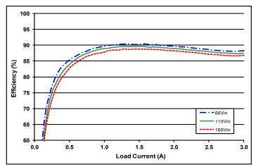
Figure 1: Efficiency at nominal output voltage vs. load current for minimum, nominal, and maximum input voltage at 25  $^{\circ}$ C.
