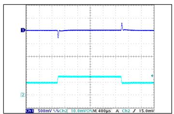
Figure 5: Output voltage response to step-change in load current (50 % -75 % -50 % of Iout(max);  $dI/dt = 0.1 \ A/\mu s$ ). Load cap: 15  $\mu F$  tantalum cap and 1  $\mu F$  ceramic cap. Ch 1: Vout, Ch 2: Iout. (10 A/div.)
